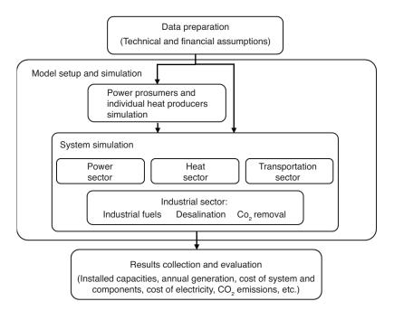
Figure 1: Fundamental structure of the LUT Energy System Transition model [16,17]
