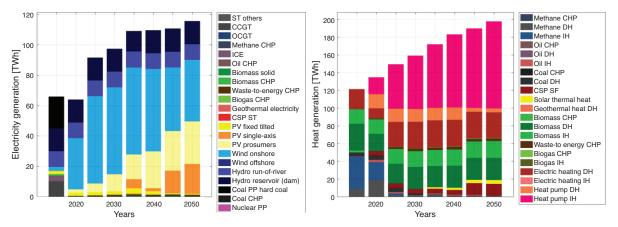
Figure 7: Power and heat - Electricity generation by power technology (left) and heat generation by heat technology (right)
