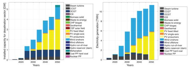
Figure 13: Desalination - Installed capacity by power technology (left) and electricity generation by power technology (right)
