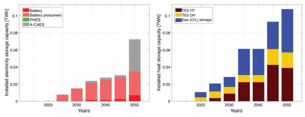
Figure 8: Power and heat - Installed electricity storage capacities (left) and heat storage capacities (right)
