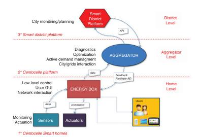
Figure 1: Connection architecture
