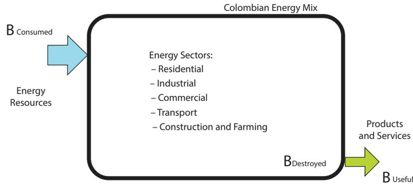
Figure 2: Control volume used for the calculation of the exergy efficiency of the energy consumption in the Colombian energy mix.
