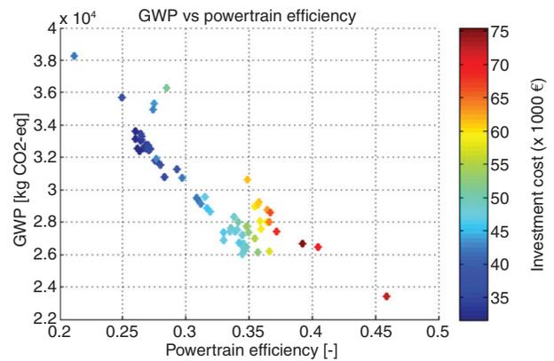
Figure 4: Pareto curve – total GWP to powertrain efficiency, investment cost in color bar, NEDC.
