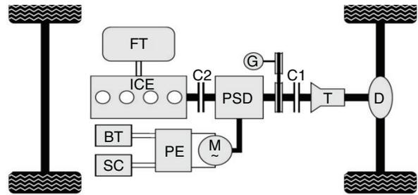
Figure 3: Parallel hybrid electric architecture: FT – fuel tank, ICE – internal combustion engine, BT – high voltage battery, SC – super capacitor, PE – power electronics, M– electric motor, PSD – power split device, G – electric generator, C1- clutch 1, C2- clutch 2, T- Transmission, D- Differential
