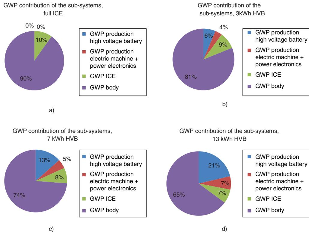
Figure 8: GWP contribution for the production phase of the vehicles sub-systems a) Full ICE, b) 3 kWh of HVB, c) 7 kWh of HVB, d) 13 kWh of HEV
