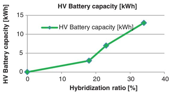
Figure 5: Correspondence between the high voltage battery capacity and the hybridization ratio.
