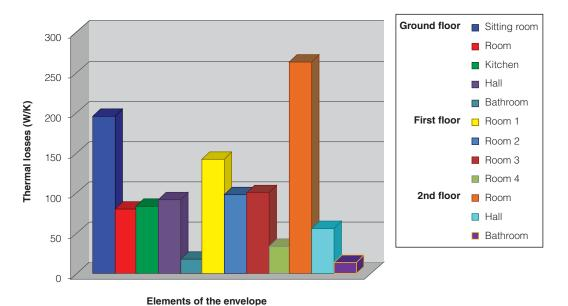
Figure 6: Losses due to heating of each room
