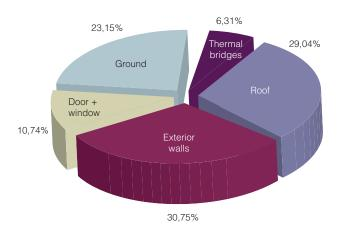
Figure 5: Share of total losses for the existing building : (a) permeable house to the air infiltration, (b) perfectly tight house.
