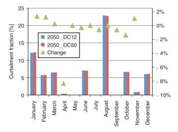
Figure 6: Curtailment fraction for off-shore wind in CC2050 with electricity demand curves from 2012 (2050\_DC12) and 2050 (2050\_DC50). Note, the change between the curves shown along the right axis is not in percentage point but in percent.
