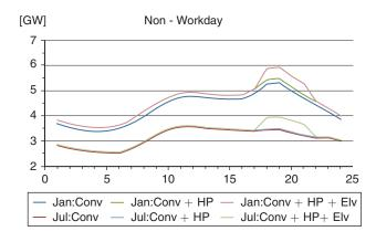
Figure 4: Effects on the hourly demand from the introduction of individual heat pumps (HPs) and electrical vehicles (EVs) charged after work in 2030.
