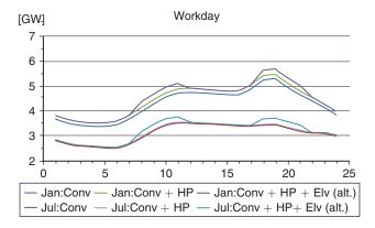
Figure 5: Effects on the hourly demand from allowing half of the electrical vehicles to be charged at work (EV(alt)) in 2030.
