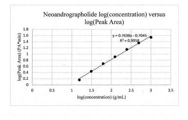
Figure 8: Calibration Curve for Neoandrographolide.
