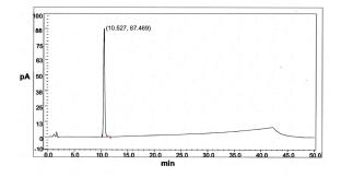
Figure 2: HPLC Results for Andrographolide Standard (1 mg/mL).
