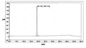
Figure 3: HPLC Results for Neoandrographolide Standard (1 mg/mL).
