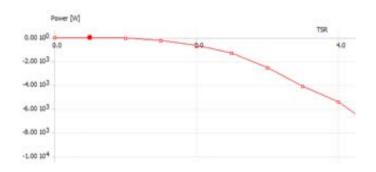
Figure 13. Output power at different tip speed ratios.
