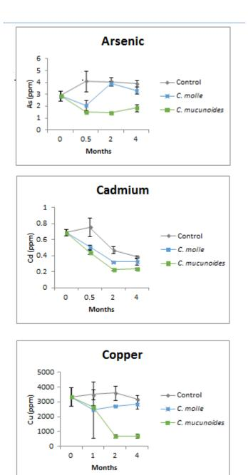
Figure 3. Reduction of As, Cd, and Cu concentrations in mine tailings before and after the experiment. Values indicate Mean  $\pm$  SE; n = 3; in parts per million.
