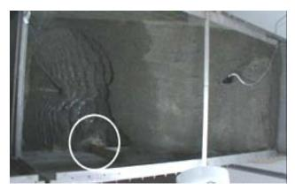
Figure 3. Piping at the toe of the slope model (view from Camera 2).
