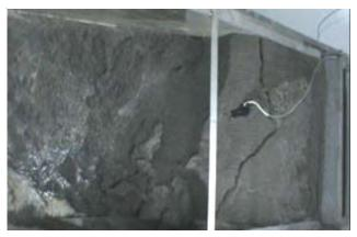
Figure 5. Plan view of the largest tension crack just above the upslope sensor column. (view from Camera 2).
