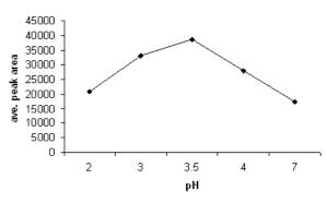
Figure 1. Average peak areas (n=3) for 10  $\mu g \ L^{-1} \ BrO_3^{-} at$  varying pH of the mobile phase.
