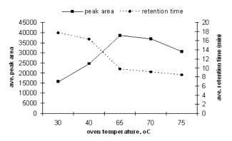
Figure 2. Average peak areas (n=3) and retention times (n=3) for 10  $\mu$ g L<sup>-1</sup> BrO<sub>3</sub><sup>-</sup> at varying oven temperatures in °C.
