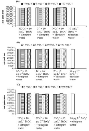
Figure 3. Comparison of inorganic anions [(A):  $HCO_3^{-}$ ,  $CI^{-}$ ,  $NO_3^{-}$ ; (B):  $SO_4^{2-}$ ,  $Br^{-}$ ; (C):  $NO_2^{-}$ ,  $PO_4^{3-}$ ,  $CIO_3^{-}$ ] at different concentrations spiked in ultrapure water containing 10 µg L<sup>-1</sup> BrO<sub>3</sub><sup>-</sup> and ultrapure water containing 10 µg L<sup>-1</sup> BrO<sub>3</sub><sup>-</sup> only.
