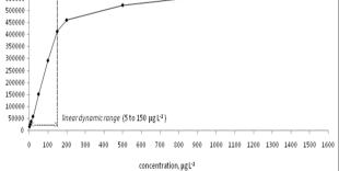
Figure 4. Graphical representation of the peak area response of 2 to 1500  $\mu$ g L<sup>-1</sup> BrO<sub>3</sub><sup>-</sup> (n=3) in ultrapure water showing linear dynamic range.
