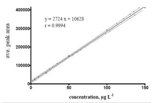
Figure 5. A linear calibration graph for 2 to 150  $\mu$ g L<sup>-1</sup> BrO<sub>3</sub> solutions (n=3) using the optimized ion chromatographic method. [Solid line represents linear regression and dotted lines show 95 % confidence interval levels about the regression.]
