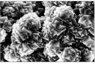
Fig. 6. Enlarged SEM image of  $MgB_2$  film deposited for 2 min.
