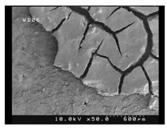
Fig. 1. MgB<sub>2</sub> film deposited on silver substrate.
