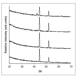
Fig. 3. XRD patterns of MgB, deposited on Mo by EPD.
