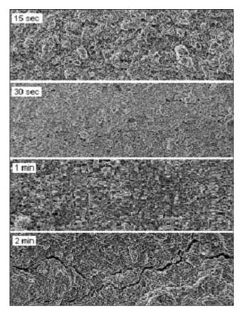
Fig. 2. Deposition surface of  $MgB_2$  films (400x).
