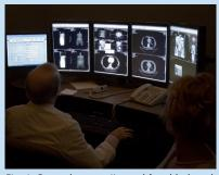
Fig. 4. One colour monitor and four black-andwhite monitors. Note the differences in height between the displays and the input devices (mouse and keyboard).
