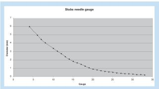
Fig. 1. Needle gauge versus outer diameter in mm. Inner diameter ranges from 40% (smaller gauges) to 80% (larger gauges) of outer diameter.
