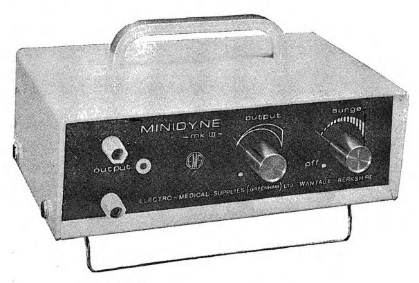
Representing another advance in the evolution of the Minidyne, the Mark III version incorporates printed circuits which reduce the size but also enhance the reliability; continuing features are
