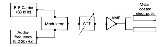
Fig 1: Schematic of high-frequency audiometer (From: Tonndorf and Kurman, 1984)
