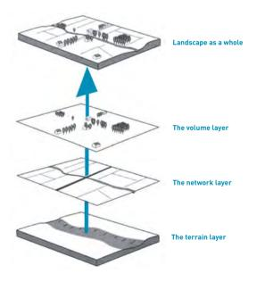
Figure 4 A visible landscape representation (source: Wassink, 1999) On bottom the DEM (terrain layer). Successive layers like network (line and area objects) and volume layer (3D objects) put forward a DLM (on top) ings, trees and other artifacts, a DLM will be created out of the DEM. For example a 2D georeferenced elevation dataset, like the Dutch AHN, can be supported by a selection of vertically extruded 2D objects to generate a DLM out of a DEM as presented in figure 6.
