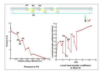
Fig. 8. Pressure and local heat transfer coefficient for staggered ripsaw fin with thickness 0.0005 m
