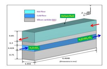
Fig .1. Geometry and dimensions of the channel
