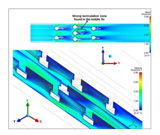
Fig .5. Velocity streamlines for the single channel model with staggered rectangular fins at y=0.003 m and z=0.0048  $\,$  m
