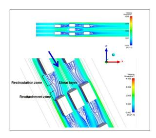
Fig .2. Velocity streamline for single channel model with staggered rectangular fins along y-plane at y=0.003 m and bottom solid regions
