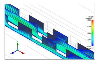
Fig. 3. Velocity streamline for single channel model with staggered rectangular fins along z-plane at z=0.0015 m
