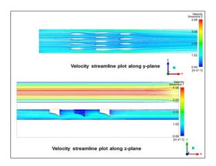
Fig .7. Velocity streamline for single channel model with staggered ripsaw fin with thickness of 0.00005 m at y=0.0037 m and z=0.0047 m
