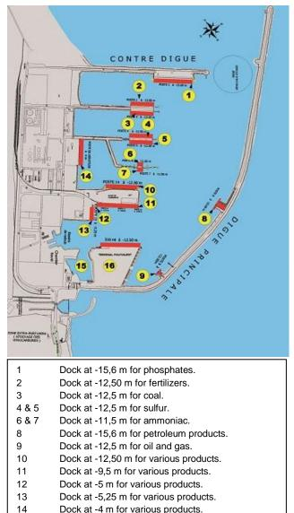
Fig .2 Jorf Lasfar port caracteristics and connectivity.
