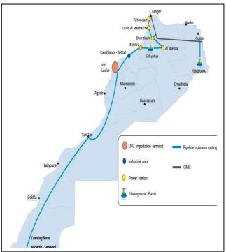
Fig .10 Optimum routing solution.
