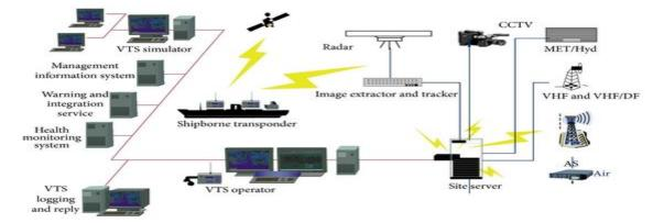
Fig .4. System architecture of VTS service.
