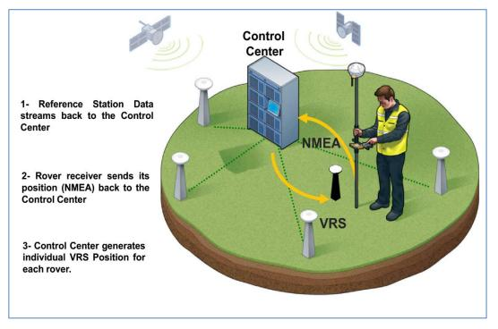
Fig .4. Virtual Reference Station concept
