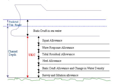
Fig .9 Factor allowances associated with a Gross UKC Calculation [10]
