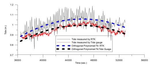
Fig .6 Tide values measure by the tide gauge and by RTK GPS [3].
