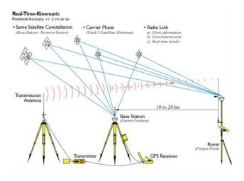
Fig .3. Real Time Kinematic GPS technique
