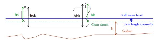
Fig .10 GPS concept for monitoring ship UKC [7]
