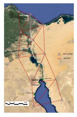
Fig .11 The proposed GNSS network in Suez Canal Corridor Area
