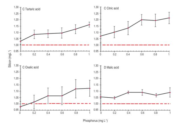
Figure 2. Silicon concentrations (mg L<sup>-1</sup>) determined in the presence of increasing concentration of phosphorus and four organic acids (at 0.8 mg L<sup>-1</sup>): A Tartaric acid, B citric acid, C oxalic acid, and D malic acid.
