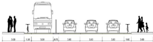
Figure 6. Road section and position of bicycle lanes as a result of rearrangement of the central ring route
