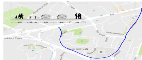
Figure 7.4. Road: Ilijaz Kodra (route and road section)
