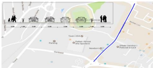
Figure 7.9. Road: Zahir Pajaziti – Nënë Tereza Boulevard (route and road section)
