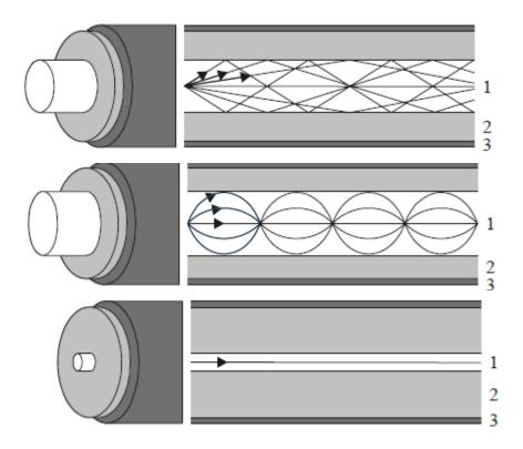
Fiber in the first image is called "scale fiber" as fleeting changes refraction index from the middle layer in core. As a result, all rays (modes) within a certain angle will be reflected fully in the boundary core-middle layer. From this we see that the modes reach the end of fiber at different times causing signal limites to be broadcast.
