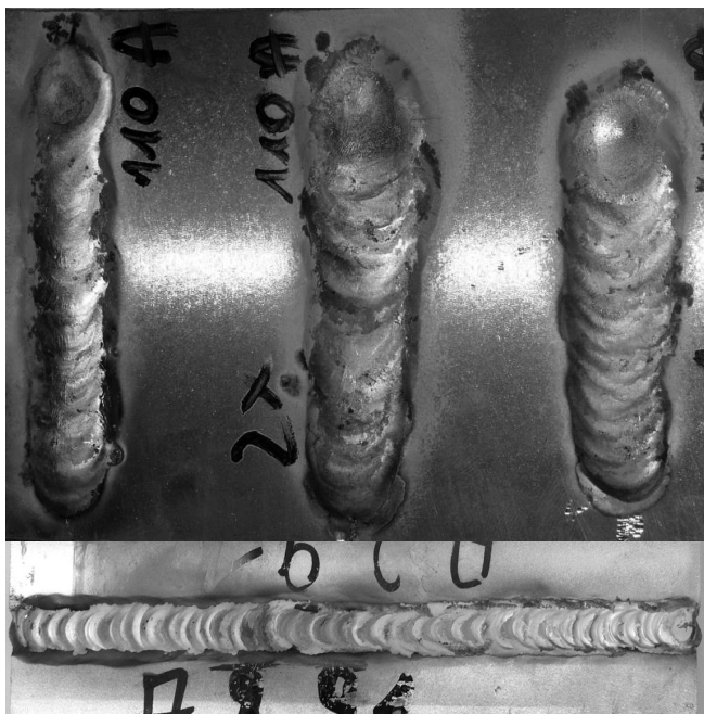
Rys. 1. Złącza spawane i napoiny odlewniczego stopu magnezu AZ91 – widok od strony lica Fig. 1. Joints and pad welds in magnesium alloy AZ91 casting alloys – view from the face
