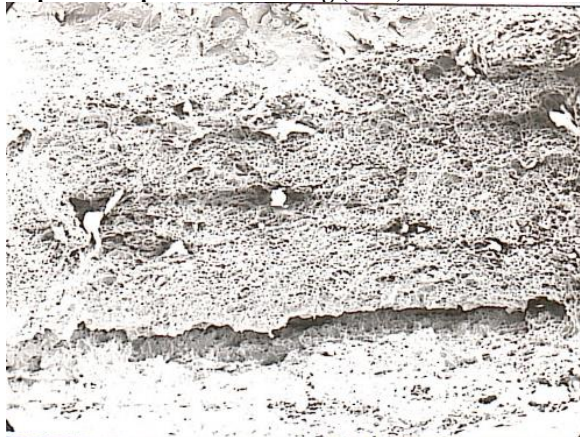
Fig. 5. Fractogram of the surface with surfacing composite coating CCCM. Base - steel 45 The results of tests of brake pads for cyclic (long-term) strength are shown in Figures 6 and 7.
