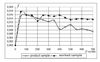
Fig. 3. Dependence of friction coefficient on working life at volumetric temperature of oils  $20^{\circ}\mathrm{C}$
