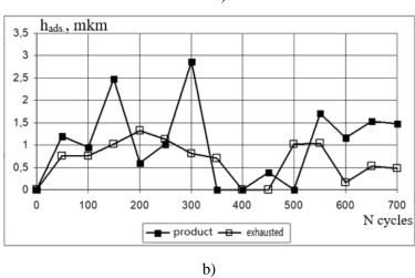
Fig. 1. Dynamics of formation of boundary adsorption layers (had.) with Mobil-1 oil at  $20^{0}C$  (a) and  $120^{0}C$  (b) at operating time (N)
