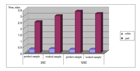
Fig. 4. Linear wear of the Cane friction surfaces (roller - shoe) at 700 operating cycles at volume temperatures of the lubricant  $20^{\circ}$ C and  $120^{\circ}$ C
