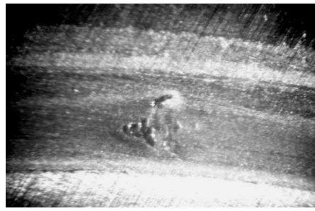
Friction track of a sample made of 40X steel without heat treatment 12 hours of work
