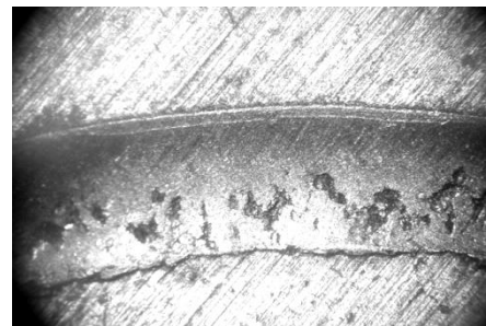
Friction track of a sample made of 40X steel without heat treatment 12 hours of work
