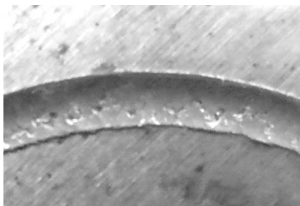
Friction track of a sample made of 40X steel without heat treatment 12 hours of work
