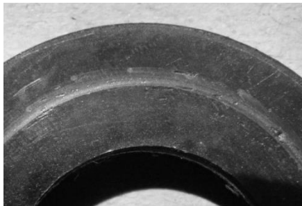
Friction track of a sample made of 40X steel without heat treatment 12 hours of work
