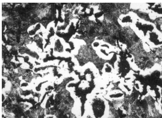
Fig. 9. Microstructure of microalloyed chromium CIVG after MICF (cross section of casting with a thickness of 35 mm);
