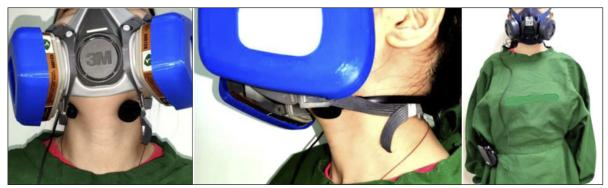
Figure 2. Laryngophone receivers positioned at the level of the hyoid and speaker attached to the protective gown.
