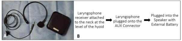
Figure 1 A. Laryngophone and speaker; and B. Schematic outline of set-up Device Set-up
