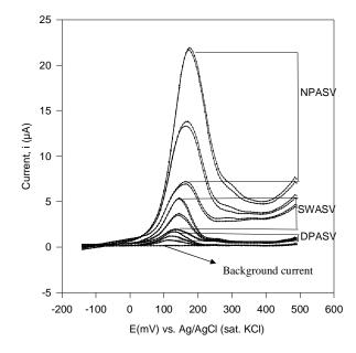
Figure 1: Comparison between three different electroanalytical methods for  ${\rm As}^{3^+}({\rm same}\ {\rm concentration})$  at solid gold electrode.
