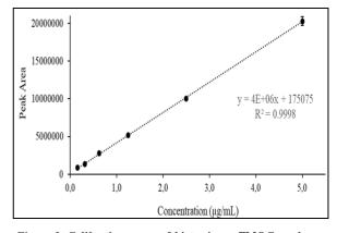
$\label{eq:Figure 3.} \textbf{ Calibration curve of histamine} - \textbf{FMOC}, \ \textbf{peak area} \\ \textbf{versus concentration}$
