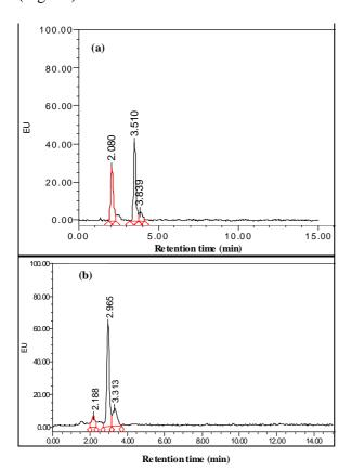
Figure 4. (a) The chromatogram of histamine standard derivatized by FMOC-Cl (ex: 267/ em: 314) and (b) the chromatogram of mackerel derivatized with FMOC-Cl (ex: 267/ em: 314)
