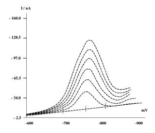
Fig. 2. Cathodic stripping voltammogram for CFL indicating potential (mV) verses current (nA) in 20% methanol plus 80% 0.1M HCl plus 0.1 M KCl, pH 4.0, concentrations 1, 10, 20, 30, 40, 50  $\mu$ g/ mL, peak potential -0.75 V.
