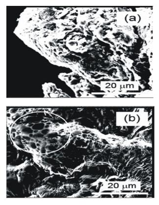
*Figure 1.* FIB/SEM images of (a) Ca-Alg<sub>2</sub> and (b) Ca-Alg<sub>2</sub>/GO gel beads after drying in molten naphthalene. Circled image in (b) indicates more defined porous structures in Ca-Alg<sub>2</sub>/GO gel beads (b), circled have pore sizes ranging from 1 to 5  $\mu$ M. [18] Reproduced with permission from publisher. Source.
