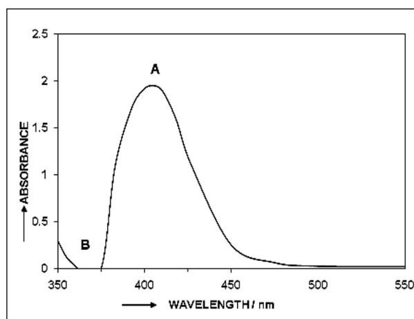
Figure 1. A and B absorption spectra of Cu<sup>II</sup>- Sal-BH system ( $\lambda_{\text{max}} = 404\text{nm}$ ) and the reagent blank, respectively in aqueous solutions.
