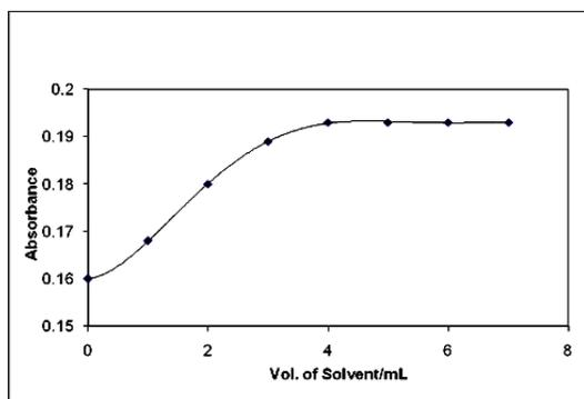
Figure 2. Effect of solvent on the absorbance of Cu<sup>II</sup>-Sal-BH system.
