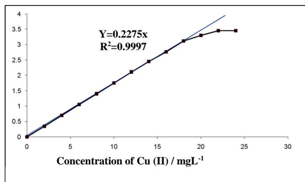
Figure 5. Calibration graph, 1-18 mgL<sup>-1</sup> of copper(II).
