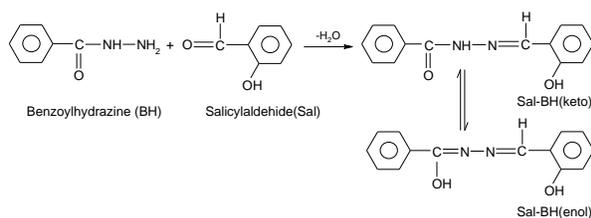
Reaction scheme of salicylaldehydebenzoylhydrazone(Sal-BH)
