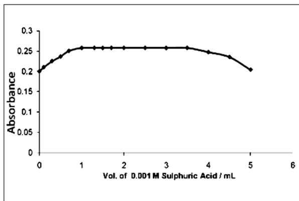
Figure 3. Effect of the acidity on the absorbance of Cu<sup>II</sup>-Sal-BH system.
