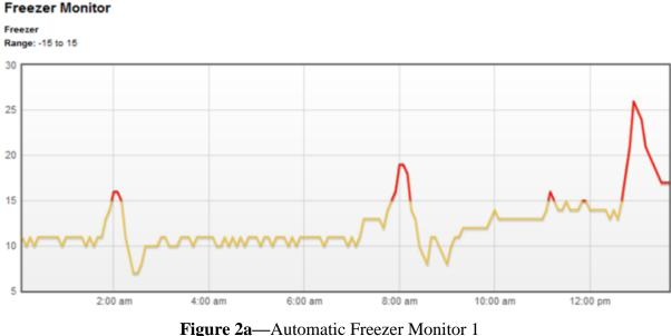
**Figure 2a**—Automatic Freezer Monitor 1 Color code: Yellow = normal range, Red = above normal range
