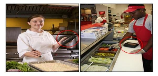
Figure 3. Automatic Handheld Probes for Temperature Collection and Transmission
