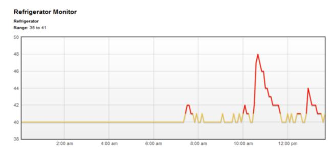
**Figure 2b--**Automatic Refrigerator Monitor 2. Color code: Yellow = normal range, Red = above normal range
