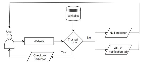
Figure 3: Flow diagram of proposed AHT2 extension whitelisting algorithm
