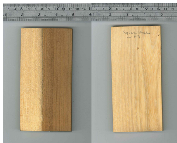
FIGURE 3: Quarter-sawn timber showing sapwood and heartwood labelled S. microphylla (left) and sapwood timber labelled S. tetraptera (right), from the New Zealand School of Forestry’s historic wood collection.
