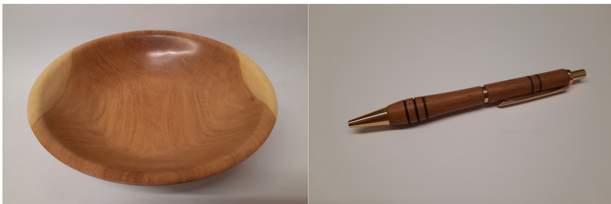
FIGURE 7: Decorative bowl turned from Sophora spp. heartwood and sapwood (left) and pen turned from Sophora spp. heartwood by Dave Page (Scion).
