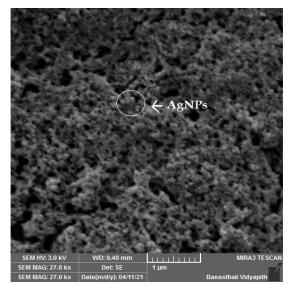
Figure 7. Scanning electron microscopy of synthesized AgNPs using *Delonix regia* shoot extract
