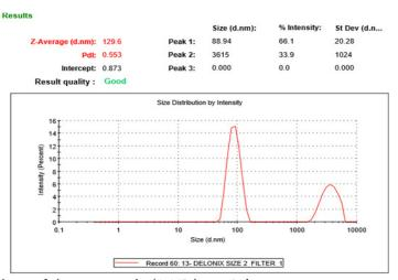
Figure 4. Particle size of silver nanoparticles (AgNPs)using Delonix regia
