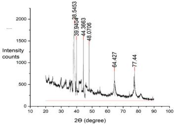
Figure 3. X-ray diffraction pattern of AgNPs using Delonix regia shoot extract
