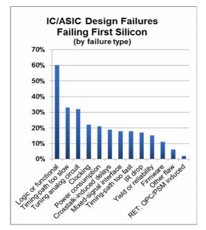
Figure 1. Failure types on the first silicone.
