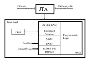
Figure 10. Design diagram of FPGA-based embedded system.
