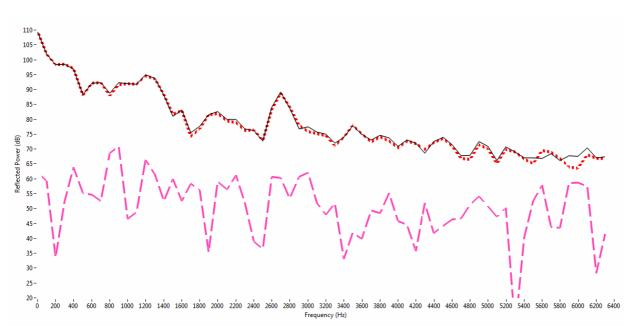
Fig. 5. Spectra of land clutter (solid – 1<sup>st</sup> period spectrum, points – 2<sup>nd</sup> period spectrum, dashed – difference)
