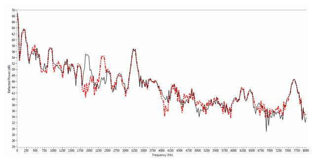
Fig.3. Spectra of clutter and moving targets (solid – up- spectrum, dashed – down- spectrum)
