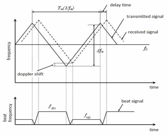
Fig. 1. FMCW triangular waveform and beating signal
