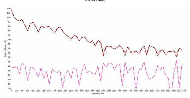
Fig. 6. Spectra of land clutter with a layer of 10 cm snow (solid – 1<sup>st</sup> period spectrum, points –
