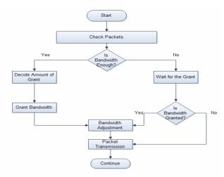
Fig. 4. Algorithm of Controlled DBA
