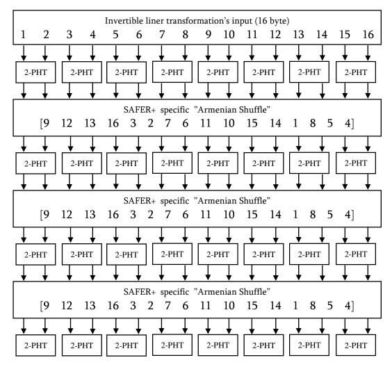
Fig. 1: Invertible linear transformation layer of SAFER+.
