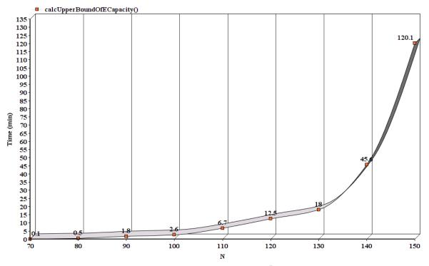
Fig. 5. Performance of calcUpperBoundOfECapacity() function for various N when Advanced Inftheo is in MPI mode with usage of 40 processors.
