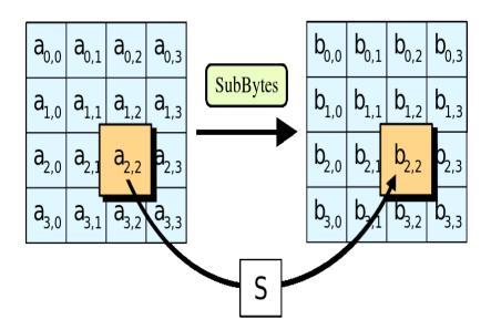
Fig. 2. AES subbytes operation.
