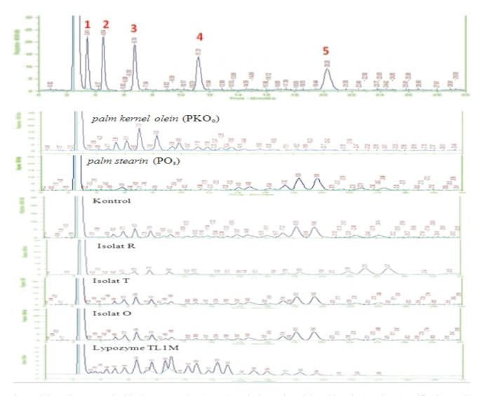
Fig 9 High Performance Liquid Chromatography (HPLC) analysis result. Triglyceride Mix Standart; Specification peak: [1]Glyceryl trioctanate; [2]Glyceryl tridecanoate; [3]Glyceryl tridodecanoate; [4] Glyceryl trimyristate; [5]Glycerol tripalmitate.
