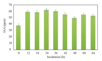
Fig 6 IAA production by by *Acinetobacter* sp. during scale up production of IAA with mung bean sprout extract as precursor in the 20 L fermentor. The experiments were performed in triplicates and the bars indicate standard deviations.
