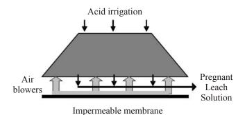
Fig 2 Schematic of a heap leaching operation.
