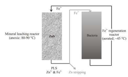
At present, all biomining operations use sulfide ores, and metals are recovered by a process of oxidative dissolution of metal-bearing minerals. Some metal ores, however, are already oxidized (such as nickel laterites,
