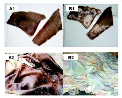
Fig 8 Application of proteases from *B. megaterium* DSM 319 in dehairing of cow hide. A: raw hides, B: dehaired hides; A1 & B1: at our laboratory; A2 & B2 at Sumber Kulit in Magetan, East Java.
