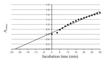
Fig 5 Protease hydrolyzed specific chromogenic substrate for trypsin, Y = 0.024 t + 0.664, R2 = 0.971.
