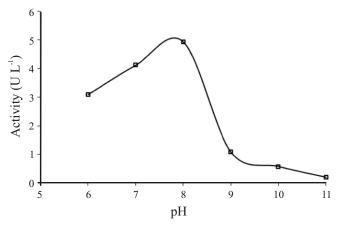
Fig 2 Effect of pH on proatease activity at 30 °C in universal buffer.
