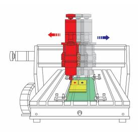
Figure 4. Machine path on making markings
