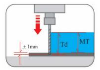
Figure 6. Tool depth in making the markings
