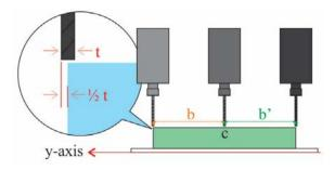
Figure 10. Guidance on making the two markings on y-axis
