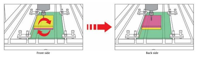
Figure 7. Flipping material to do back-side machining
